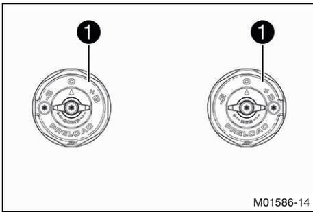
Cartridge article number ❶ is located on the side of the screw cap.
