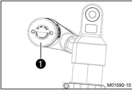
Shock absorber article number **1** is located on the bottom of the compensating tank.
