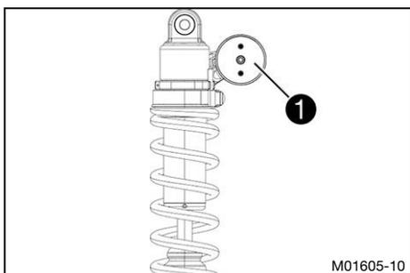
Shock absorber article number ❶ is located on the bottom of the compensating tank.
