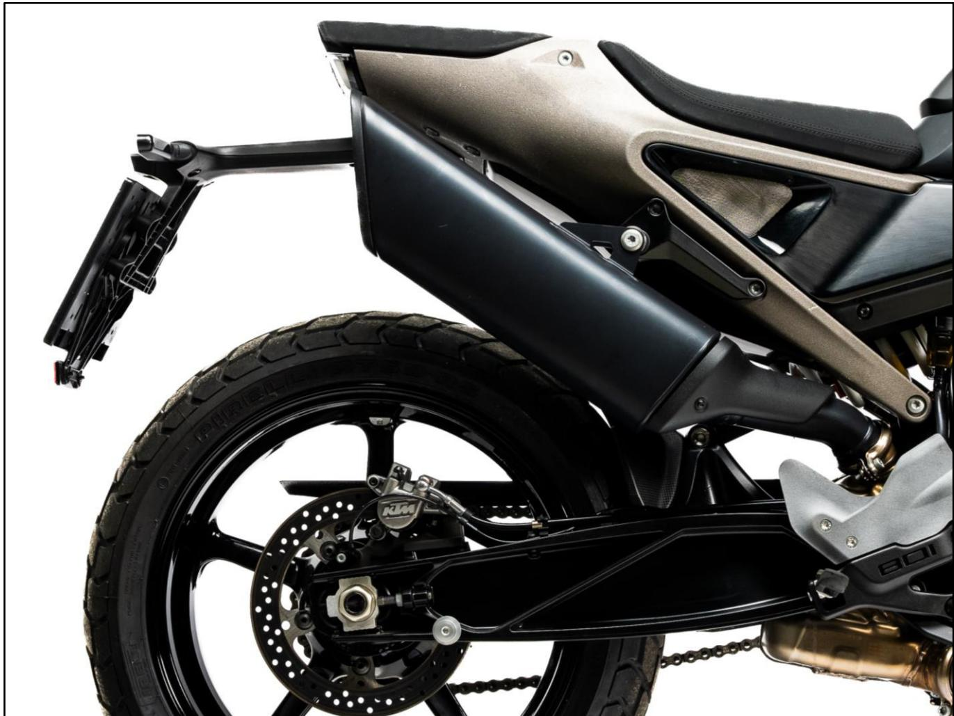
Take off the serial muffler by loosening the clamp and bracket screw.
