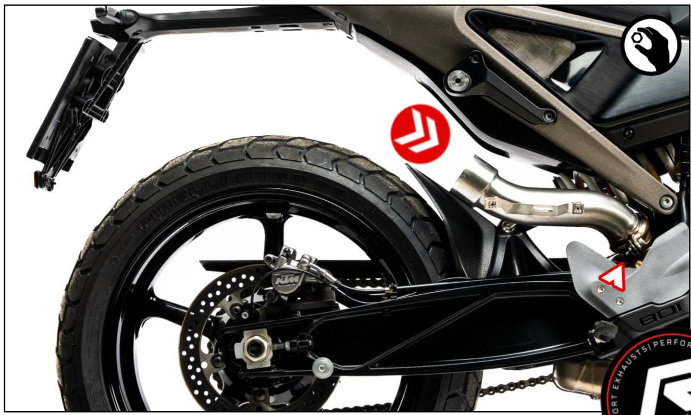
Slip on the REMUS sport exhaust onto the connection tube, screw the bracket and hook the spring.
