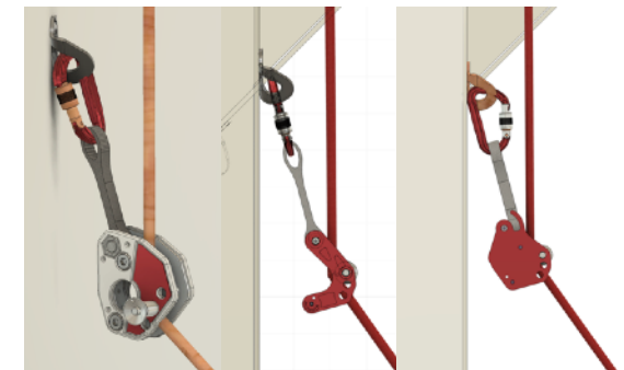
Fig. 8: Correct clipping orientation of ZAED / ZAED mini / ZAED pro to the wall
