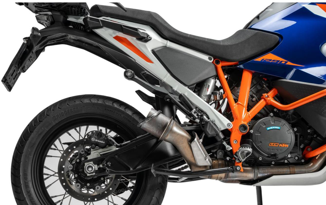
Slip on the REMUS sport exhaust onto the serial header, use the serial clamp and gasket.
