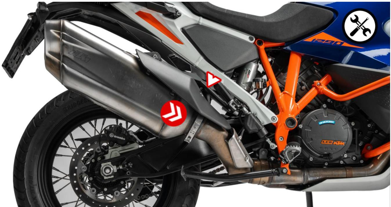
Loosen the screw of the bracket as well as the clamp and remove the serial muffler.
