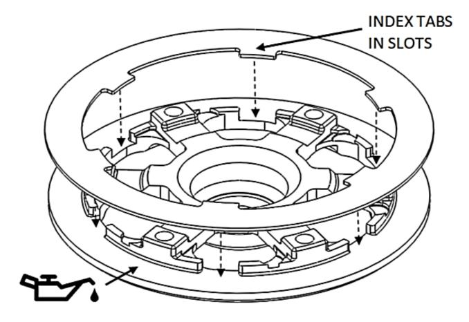
11. Install this pressure plate / lining plate combo, keeping the lining plate against the pressure plate. Hold the pressure plate against the clutch pack until it is bolted down in the later steps
