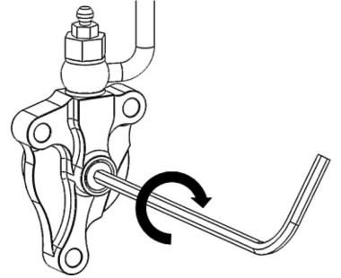
2. Once you have found the starting point, turn the adjuster clockwise 1 full turn plus 5 marks (or "1+5"). **This is NOT your final setting**, but it is a good reference point for using Free Play Gain to find the correct setting.
