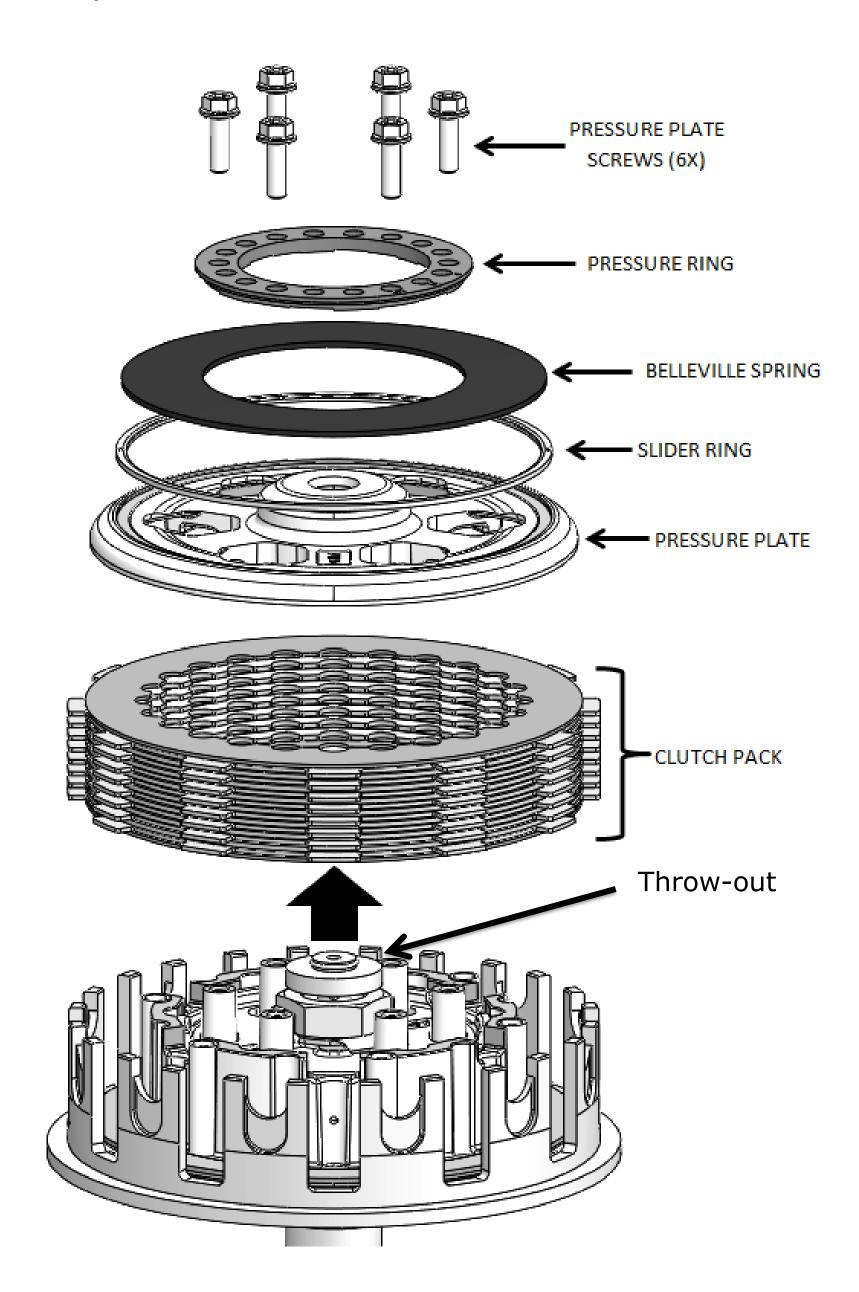
The KTM DDS clutch (a.k.a. Belleville spring clutch) employs a 2-piece damped center hub assembly, as shown. Rekluse clutch products employ the same technology and reuse the OEM rubber dampers.
