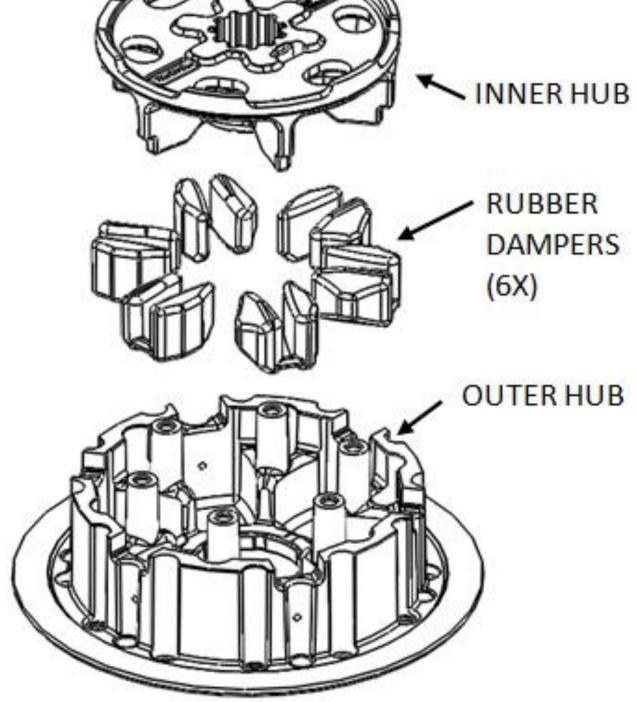
Over time, the rubber dampers will shrink due to heat and use. When this shrinkage occurs, the rotating action between the two hubs becomes loose or sloppy. This can cause hammering between the clutch parts which will reduce the life of the clutch.
