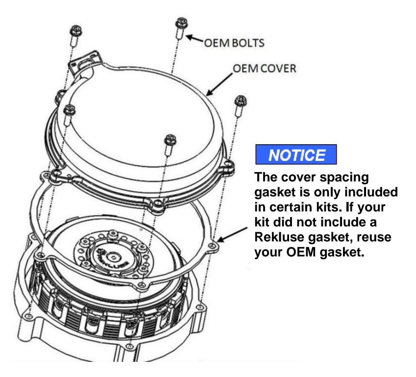
17. Install the clutch cover bolts in their proper OEM location. Lightly tighten the cover bolts in a star pattern. Torque the bolts in small increments before
