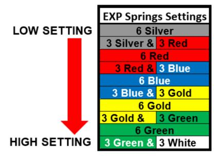
It is **NOT necessary** to disassemble the EXP halves to change springs! To change springs, remove 3 of the ¼-turn pins from one side of the EXP, replace springs, and reinstall ¼-turn pins. Next, flip the EXP disk over and repeat on the other side if necessary. To maintain even pressure when using two different color spring sets, install one color set of 3 on one side of the EXP and the remaining color set of 3 on the other side.
