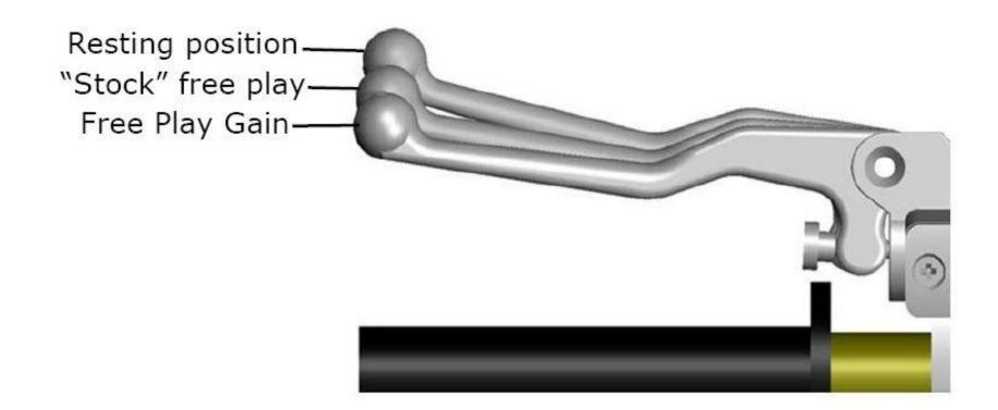
**Optimal Free Play Gain yields 1/8-1/4" (3mm-6mm)** of clutch lever movement, measured at the end of the lever. This measurement at the lever correlates to achieving the ideal installed gap.
