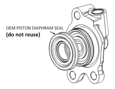
**NOTE:** When installing case sealing O-ring seal (OEM or Rekluse supplied) ensure it is seated against slave cylinder flange.
