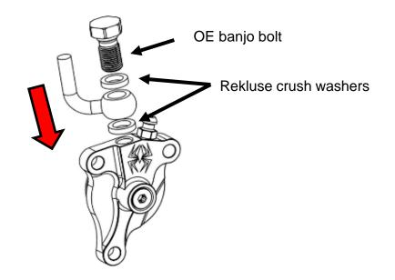
**NOTE:** A quick transfer of the fluid line will result in less bleeding in the following steps.
