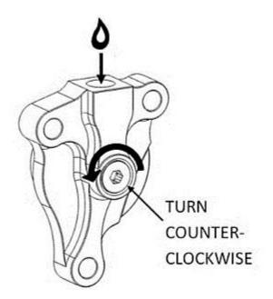
f. Compress the piston until it bottoms out. Repeat the process until there is no longer air escaping from the top port when the piston is compressed.
