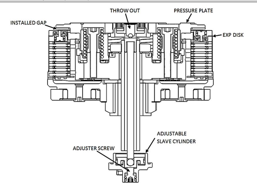
1. Using the long end of a 4mm Allen key, turn the adjuster screw clockwise until it stops under moderate pressure. You are trying to feel for the point at which the throw-out will start to lift the pressure plate. This is the "starting point".
