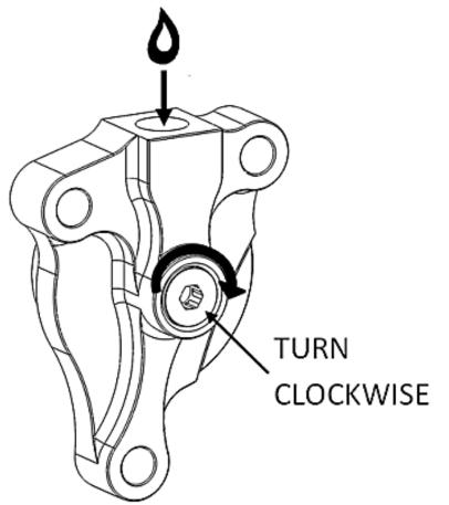
e. Turn the adjuster screw back to the initial position with the top O-ring visible.
