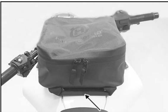
Position tank bag grip handle under the mounting plate.
