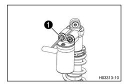
Turn the adjusting screw clockwise with a hexagon socket wrench up to the last perceptible click.
