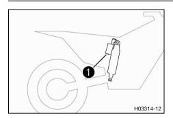
The shock absorber article number **1** is located on the bottom of the compensating tank.
