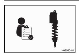
Check chassis component for damage.
