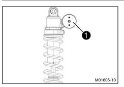
Shock absorber article number **1** is located on the bottom of the compensating tank.
