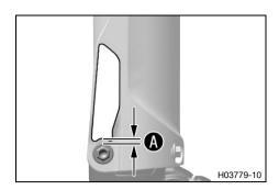
Apply the sticker for measuring sag at distance from the fork protector screw.
