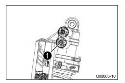
Turn adjusting screw clockwise with a hexagon socket wrench up to the last perceptible click.
