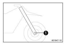
The fork article number 1 is stamped on the inside of the axle clamp.
