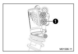
Turn adjusting screw clockwise with a hexagon socket wrench up to the last perceptible click.
