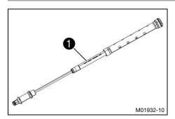
Cartridge article number 1 is located on the cartridge.
