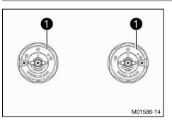
Cartridge article number  $\ensuremath{\textcircled{}}$  is located on the side of the screw cap.
